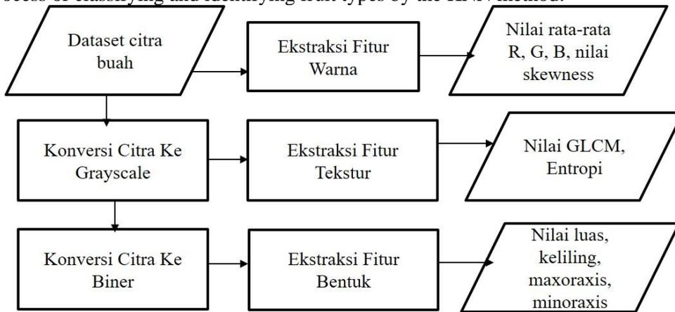
Figure. 1. Flow processing Feature Extraction
