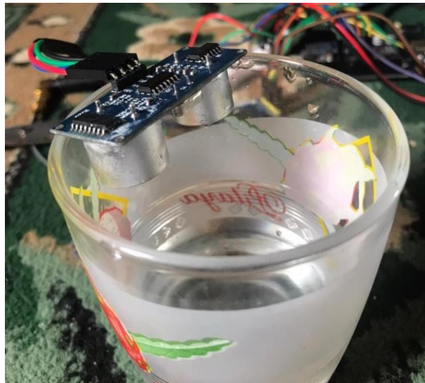
Fig. 14 Testing Process of Water Level Detetion
